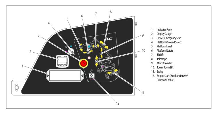
Figure 3-1. Ground Control Console
