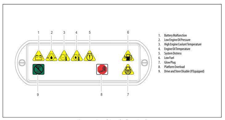
Figure 3-3. Ground Control Indicator Panel
