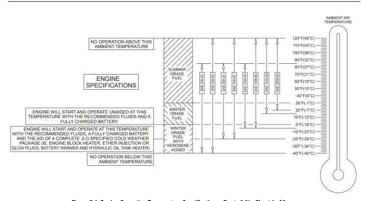
Figure 7-1. Engine Operating Temperature Specifications - Deutz 2.3L - Sheet 1 of 2
