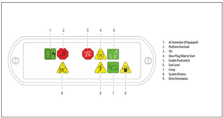
Figure 3-9. Platform Control Indicator Panel
