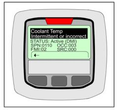
Figure 3-6. Engine Diagnostic Screen
