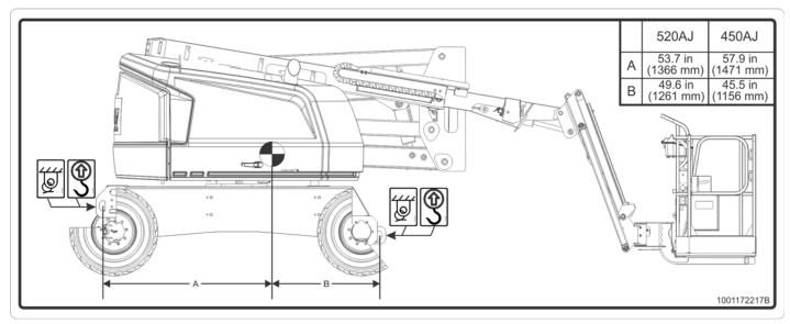
Figure 4-5. Lifting and Tie Down Chart
