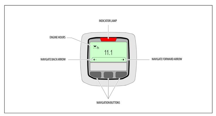
Figure 3-7. Ground Control Console Display Gauge
